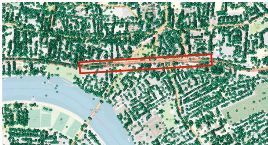
Fig. 8.11 Persistent scatterers on Hammersmith Flyover and surrounding area overlaid onto Open Street Map base imagery. Extent of Hammersmith Flyover is marked with a red box
