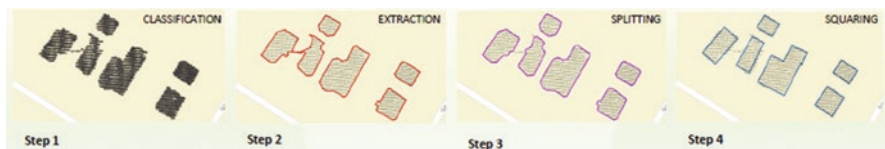
Fig. 11.2 Step-by-step method to extract building footprints from LiDAR
