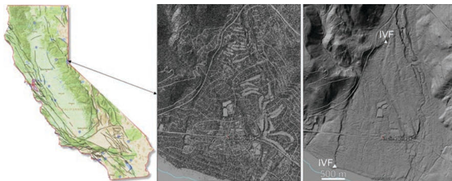
Fig. 6.6 Lidar image of Incline Village in Nevada at Lake Tahoe on the north side. Center image shows shaded relief full feature image that includes the built environment. Right image shows bare Earth model. White triangles mark the Incline Village fault (IVF) scarp. Data provided by the Tahoe Regional Planning Agency ( https://doi.org/10.5069/G9PN93H2 ) and images created by Ramon Arrowsmith for Donnellan et al. (2016)
