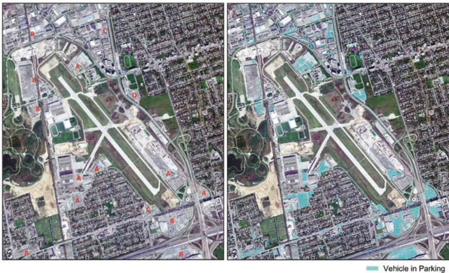
Fig. 10.6 PAN-sharpened WV3 RGB image (left) and the distribution of vehicles in parking (right) extracted from the image over a portion of Toronto. The parking lots are linked to (a) work-place; (b) retailer; (c) car dealer; (d) park-and-ride parking lot
