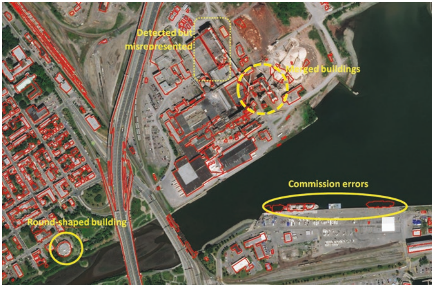
Fig. 11.3 Example of buildings from re-classified LiDAR data, including (i) detected and correctly represented, (ii) detected but misrepresented, (iii) merged buildings, and (iv) commission errors
