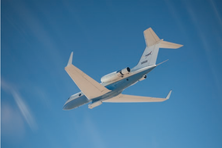
Fig. 9.2 The UAVSAR instrument is housed in a pod that mounts under the wings on the fuselage of a Gulfstream-3 aircraft. The synthetic aperture radar is a left side-looking instrument covering a ground swath 22 km wide at incidence angles extending from 22° in the near range to 67° in the far range (flat terrain values). Air ducts on the front of the pod provide ambient air cooling and a control system uses heaters to regulate the temperature of equipment in the pod. The aircraft uses a precision autopilot system to maintain its position within \pm 5 -m of the planned track. Typical operating altitude for the aircraft is 12.5 km, above normal commercial air traffic
