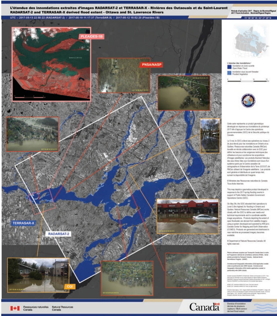
Fig. 12.4 Example of multi-sensor flood mapping using the new operational methodology from RADARSAT-2 (interior white box), and TerraSar-X (outside), showing the consistency in mapping open water and flooded vegetation between sensors
