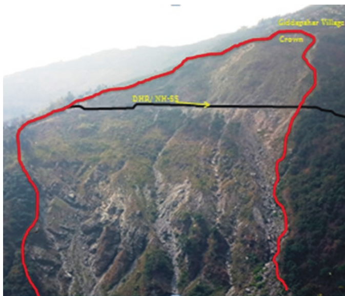
Fig. 1.4 View of the Gayabari Landslide. The Giddapahar village is situated just above the crown of the landslide. The Darjeeling Himalaya Railway (DHR)/NH-55 connecting Darjeeling district passes through the middle of the Gayabari landslide
