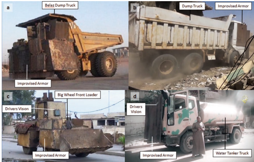
Fig. 14.3 Range of quarry and mine vehicles used by IS to make SVBIED’s in Syria and Iraq. (a) A Belaz dump truck used in mining and quarrying with an up-armoured cab driven in Syria August 2015 (Rogoway 2015; Kaaman 2019). (b) Dump truck used for moving quarry and mine spoil with an up-armoured cab driven in Anbar October 7, 2015 (Kaaman 2017). (c) Front-end loader armoured with steel plates; used as a SVBIED in NW Mosul on 15 March 2017 (Rogoway 2017). (d) Water tanker truck SVBIED used by IS in Mosul June 2014 (Kaaman 2017)
