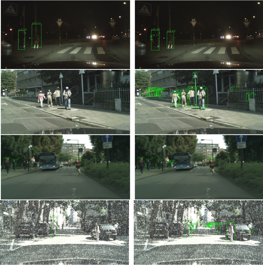
Fig. 7. Examples of detection for the baseline model and the “stylized” model (right column). The first row shows night-time detections on the ECP dataset, and the following rows show detections on the Cityscapes dataset under following corruption types (from top to the bottom): gaussian noise, motion blur, snow effect. The confidence score for each predicted bounding box is presented.
