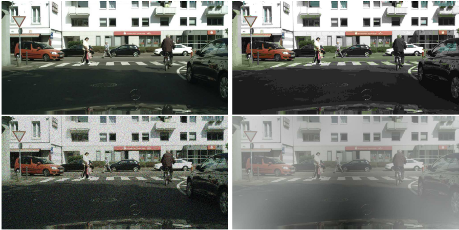
Fig. 1. Different corruption types from Hendrycks et al. Top left original image, top right - jpeg compression artifacts, bottom left - shot noise, bottom right - fog effect.
