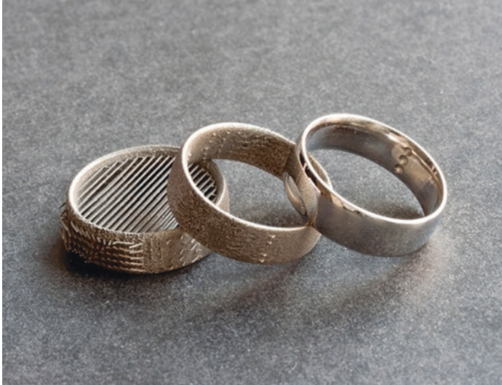
Fig. 1.5 Fabricated parts using selective laser melting: metallic part with support structures (left); part after removing the support structure (middle) and after polishing (right) (source: FH Aachen)
