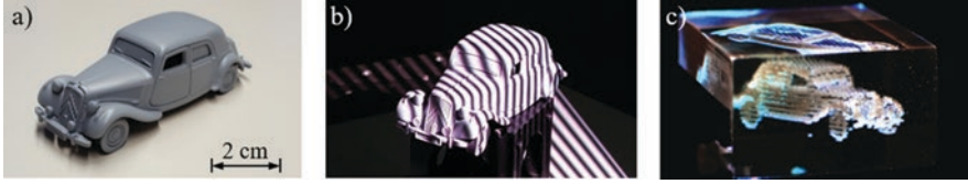
Fig. 3.49 (a) Model of an automobile with a length of 6 cm; (b) scanning process according to the binary code method with a Celluon PicoBit pico projector; (c) volumetric display with passive scattering centers in the shape of the scan template
