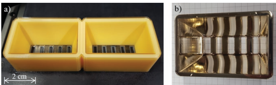
Fig. 3.53 (a) Two parabolically shaped reflectors designed to collimate the rays of an LED, currently surrounded by yellow support material after printing with the MJM process; (b) one of the reflectors from (a) after removing the support material, cleaning, and subsequent silver coating with the chemical deposition process
