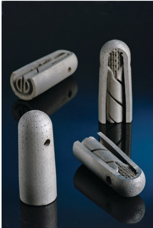
Fig. 1.18 Geometry complexity demonstrated by an interior hollow structure (source: FH Aachen)
