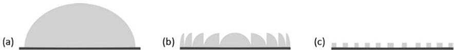
Fig. 5.22 (a) Conventional refractive lenses can be spacious along the optical axis perpendicular to the surface, depending on the curvature that is required to create the desired focal length. (b) A Fresnel lens creates the same optical function as a conventional lens but is greatly shortened along the optical axis. It has the same radius of/surface curvature as a conventional lens, while bulk material below the surface is reduced. (c) Metamaterials can be designed to show the same or even improved optical functions compared to conventional lenses. Since metamaterials consist of sub-wavelength elements (so-called metaatoms), these are ultra-flat optical elements with a thickness of 2 \mu\text{m} or smaller, for example, for VIS light
