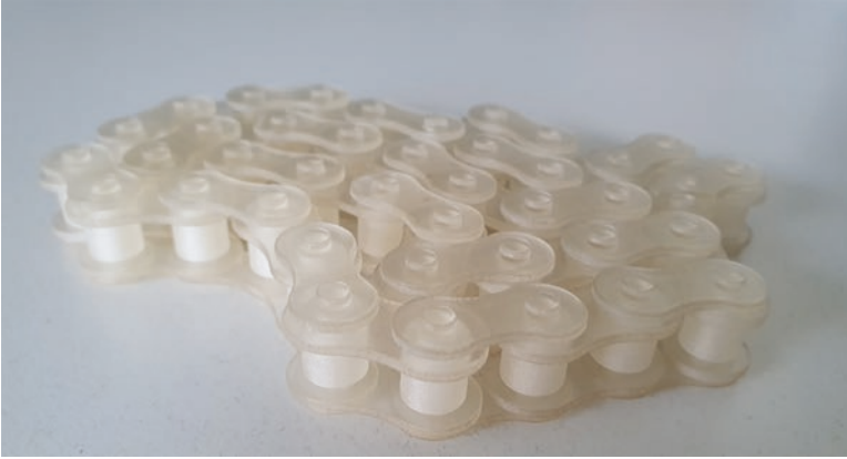
Fig. 1.3 Fabricated sample using stereolithography process (source: CP GmbH)
