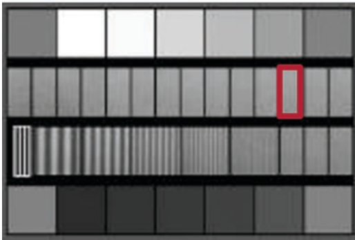
Fig. 3.33 Sine M-6 pattern with different frequencies and an image of six line pairs per mm viewed through lens no. 3
