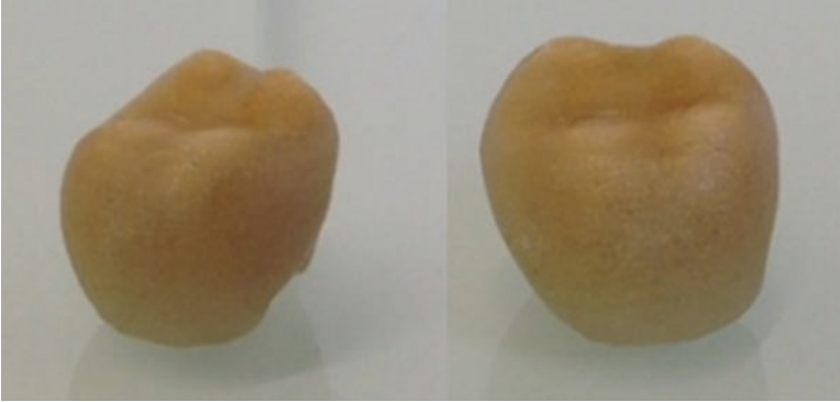
Fig. 1.7 Fabricated parts using selective laser melting of soda-lime glass [1]. (source: FH Aachen)
