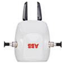
Fig. 2. A robot hand with one gripper tool and two suction cup tools
