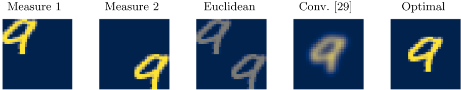
Fig. 2. Comparison among the Euclidean mean, the Convolutional Wasserstein Barycenters [29], and the optimal Wasserstein Barycenter.
