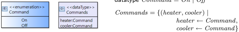
Fig. 2. Enumeration and composite datatypes in SysADL (left) and their translation to CSP (right).
