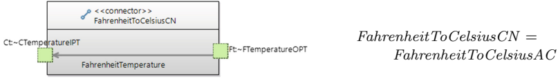
Fig. 6. Definition of a connector in SysADL (left) and its translation to CSP (right).
