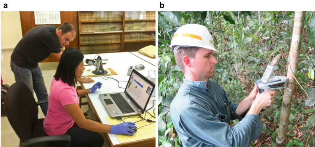
Fig. 2 a Scanning herbarium specimens using X-ray fluorescence spectroscopy (XRF) at The Sabah Forest Research Centre (FRC) in Sandakan, Malaysia, and b employing XRF technique in the field to screen for hyperaccumulator plants
