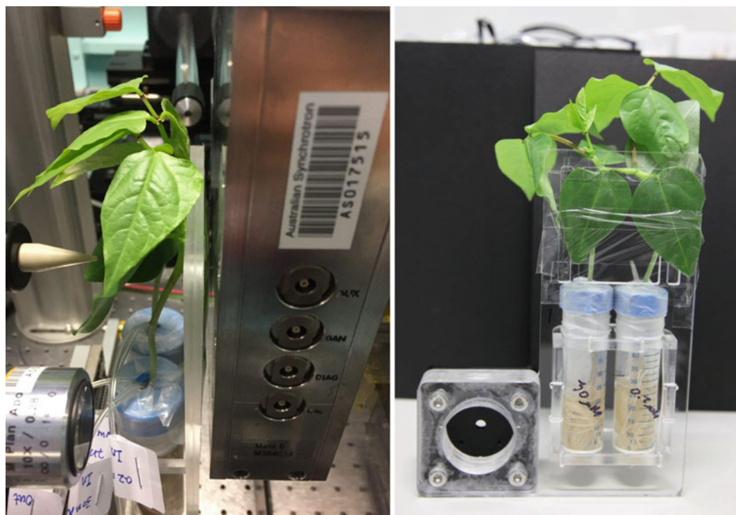
Fig. 7 Live plants (cowpea, Vigna unguiculata ) to be analyzed with the Maia detector system at the XFM beamline of the Australian Synchrotron. The leaves were scanned (4 \mu\text{m} pixels, area of 25 mm \times 5 mm) repeatedly for up to 48 h after exposure to 30 \mu\text{M} Mn
