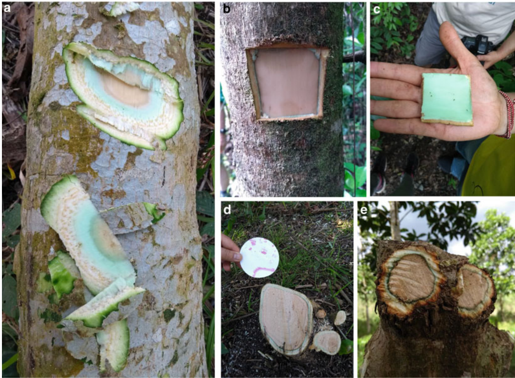
Fig. 9 a, b, e Blepharidium guatemalense tree with bright green phloem sap, and bark (c) indicative of Ni enrichment as demonstrated by a field spot test based on dimethylglyoxime (DMG) (d)
