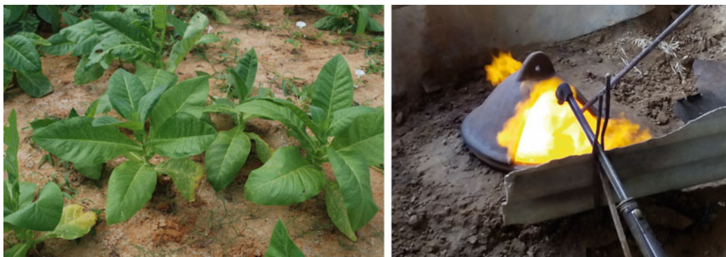
Fig. 3 Tobacco plants growing on cyanidation artisanal Au mine tailings in Lombok Island, Indonesia (left); borax smelting of the plant ash using an air-acetylene torch (right)
