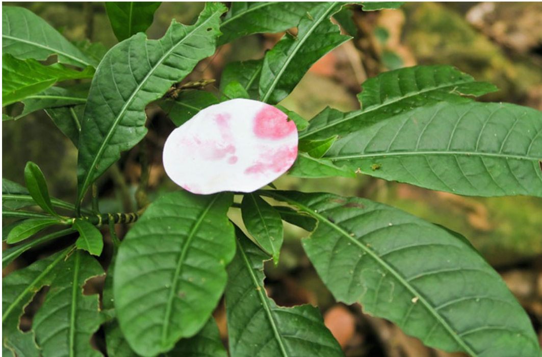
Fig. 1 Field spot test based on the Ni-specific colorimetric reagent dimethylglyoxime demonstrating the reaction with Ni from the fresh leaf of the Ni hyperaccumulator species Psychotria gabriellae
