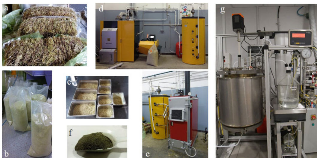
Fig. 6 Upscaling of Ni recovery from O. chalcidica : a bale of dry biomass, b ground biomass, c pellets prepared with water addition, d biomass furnace with a continuous track, e bale furnace, f ashes after combustion at 900 \text{ }^\circ\text{C} , g hydrometallurgical reactor to treat the ashes
