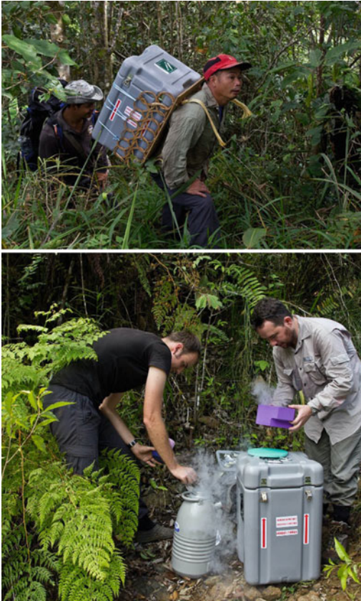
Fig. 1 Fieldwork in Malaysia: freezing samples in the field using metal-mirror fixation and transport to laboratory in a cryohipper at liquid nitrogen temperature
