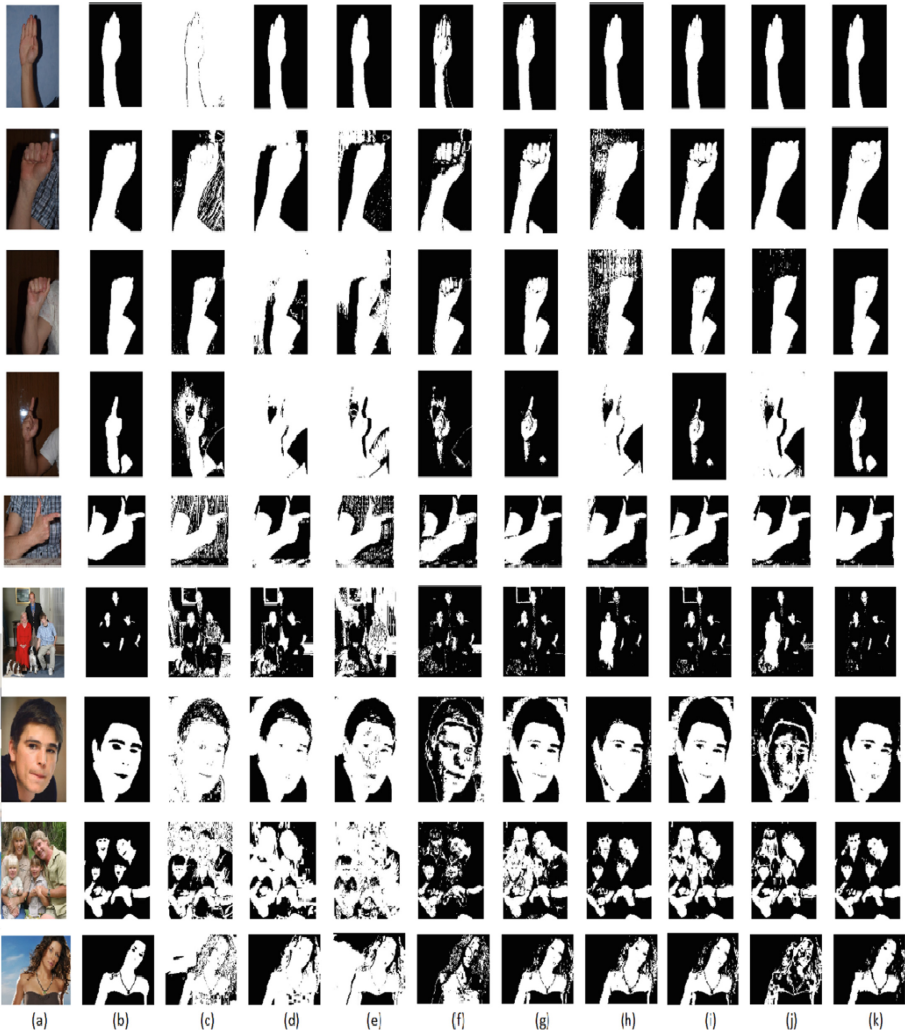
Fig. 7. Skin detection results in the two used datasets: HGR1 and Pratheepan; (a) input image; (b) skin mask; (c) Sobottka and Pitas; (d) Chai and Ngan; (e) Hsu et al.; (f) Gomez et Morales; (g) Kovac et al.; (h) Brancatti et al.; (i) RGB thresholding - S. Kolkur et al.; (j) proposed method M1; (k) proposed method M2.
