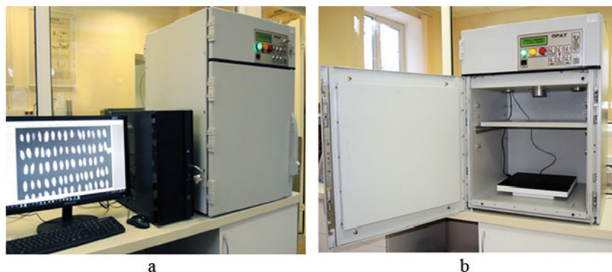
Fig. 1 The hardware-software complex for X-ray analysis of seeds of the research institute for storage of Rosrezerv: a the general type, b the upgraded X-ray unit with a digital flat-panel receiver of the X-ray image
