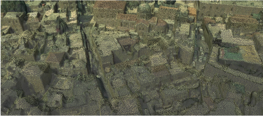
Fig. 4. Point cloud (point spacing 30 30 cm)
