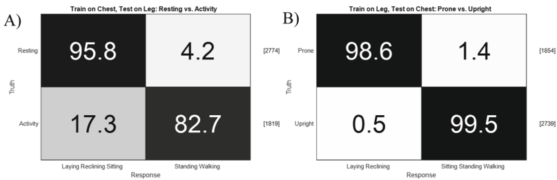
Fig. 2. Confusion matrices showing results of switching sensor locations after a classifier has been trained for the sensor placed on another location.
