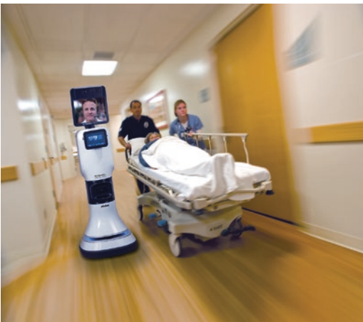
▣ Fig. 20.3 Telehealth robot. This is controlled by a remote clinician, and includes videoconferencing and remote monitoring capabilities. In this example, a specialist is connecting with a nurse during a patient transfer. Image courtesy of InTouch Health, reproduced with permission
