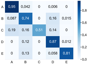
Fig. 4. Normalized confusion matrix (left) and classification metrics (right) for the activity classifier per class (A = Take probe; B = Approach Destination; C = Stand by; D = Search; E = Navigate back to base)
