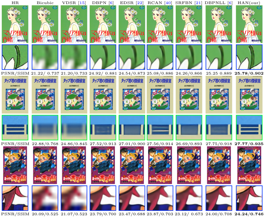
Fig. 5. Visual comparison for 8\times SR with BI model on the Manga109 dataset. The best results are highlighted
