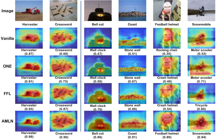
Fig. 4. The comparison of Grad-CAM [32] visualizations of the proposed AMLN with state-of-the-art methods FFL and ONE as well as the vanilla model where the peer networks use the same architecture ResNet32. The label under each heatmap is the corresponding predicted class with the highest prediction probability in the parenthesis.
