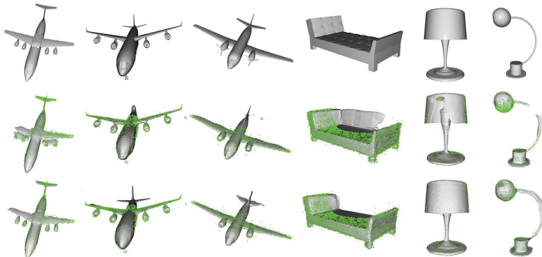
Fig. 6. The visualization results of missing part recovery. The green points are the remaining points that we use to recover the whole mesh. From top to bottom: ground truth, DeepSDF, and Curriculum DeepSDF. (Color figure online)
