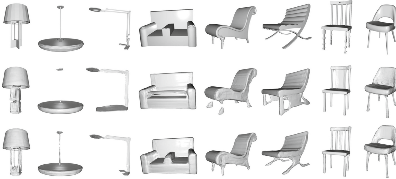
Fig. 1. 3D reconstruction results of shapes with complex local details. From top to bottom: ground truth, DeepSDF [30], and Curriculum DeepSDF. We observe that the network benefits from the designed shape curriculum so as to better reconstruct local details. It is worth noting that the training data, training epochs and network architecture are the same for both methods.
