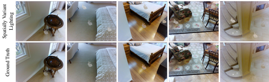
Fig. 1. Rendering examples of POINTAR in spatially variant lighting conditions. Row 1 shows the Stanford bunnies that were lit using the spherical harmonics coefficients predicted by POINTAR. Row 2 shows the ground truth rendering results.
