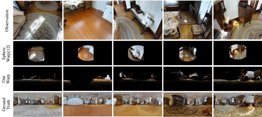
Fig. 4. Comparison of different warping methods. To transform mobile camera view spatially, i.e., from observation to warping location, we leverage the point cloud which was generated from the RGB-D image. Our approach is not impacted by distortion and therefore is more accurate than spherical warping that only considers RGB image [12].
