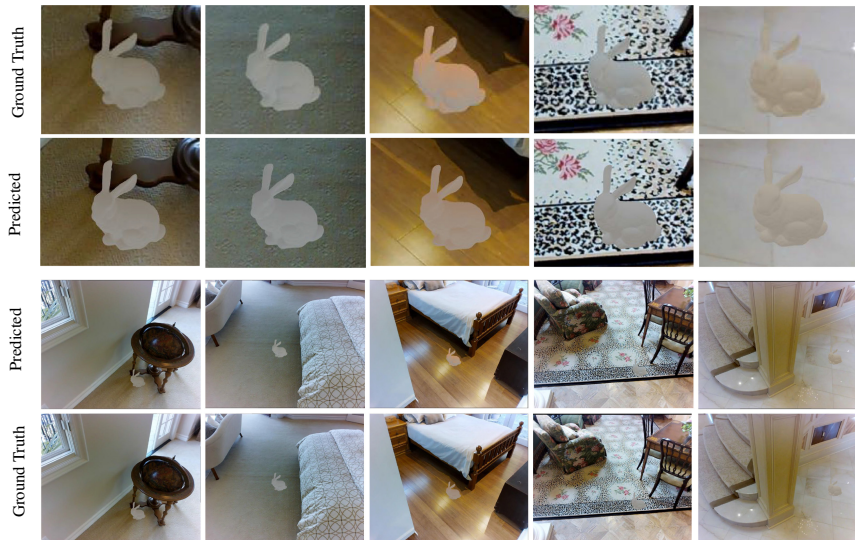
Fig. 7. Rendering example from POINTAR. Comparison between rendering a 3D object with ground truth irradiance map and irradiance map generated by POINTAR. Row 1 and 2 show the comparison between a closeup look of the rendered objects. Row 3 and 4 show the comparison between rendered objects in original observations. Note we did not cast shadow to highlight lighting-related rendering effects to avoid misleading visual effects.
