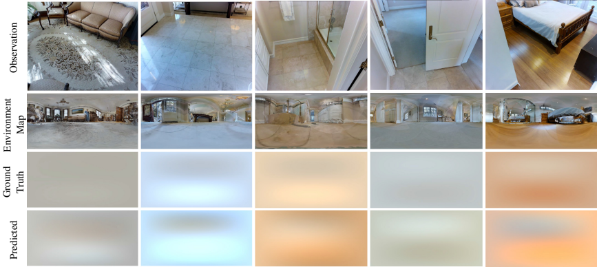
Fig. 6. Irradiance map comparison between ground truth and predicted ones. Row 1 shows the observation captured by mobile camera. Row 2 shows environment map generated from the dataset. Row 3 shows the irradiance map generated from the environment map using spherical harmonics convolution. Row 4 shows the reconstructed irradiance map from SH coefficients predicted by POINTAR.
