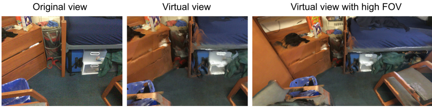
Fig. 3. Original views vs. virtual views. High FOV provides larger context of the scene which helps 2D perception, e.g., the chair in the bottom right corner is partially represented in the original view but can easily be segmented in the high FOV virtual view.
