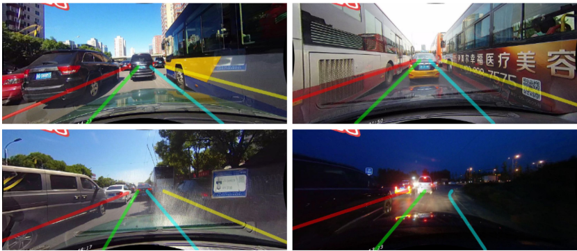
Fig. 1. Illustration of difficulties in lane detection. Most of challenging scenarios are severely occluded or distorted with various lighting conditions, resulting in little or no visual clues of lanes can be used for lane detection.
