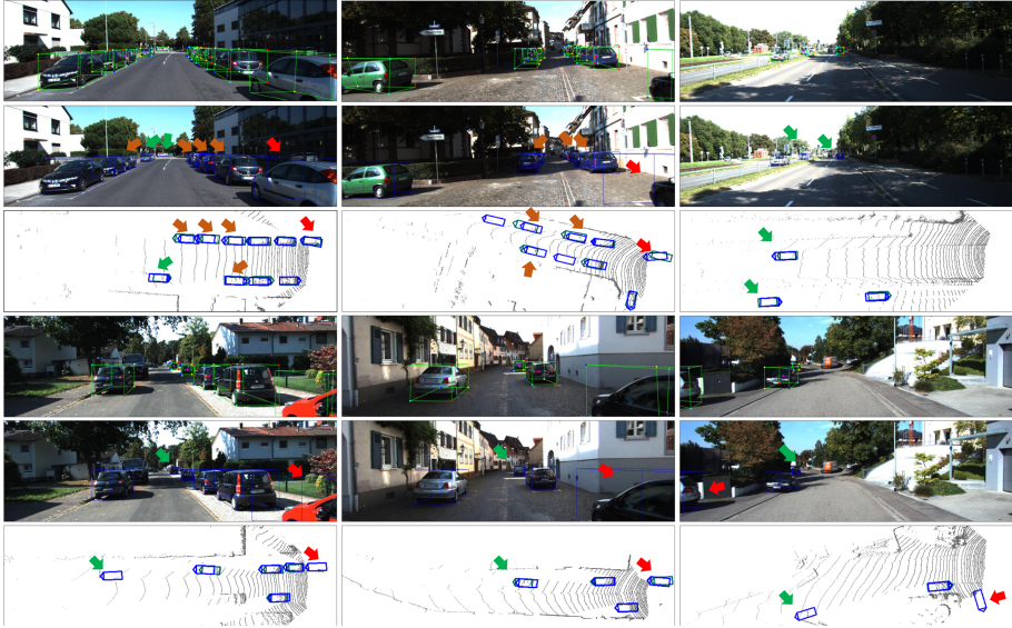
Fig. 4. Qualitative results of our 3D detection. From top to bottom are keypoints, projections of the 3D bounding box and bird’s eye view image, ground truths in green and our results in blue. The crimson arrows, green arrows, and red arrows point to occluded, distant, and truncated objects, respectively. (Color figure online)
