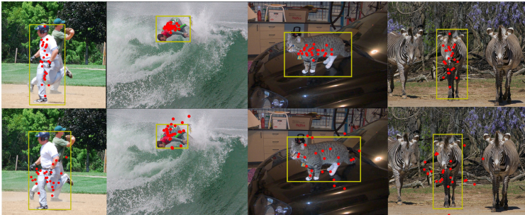
Fig. 3. MimicDet(top) vs. MimicDet w/o head-mimicking mechanism (bottom). Yellow box is the adjusted anchor box generated by refinement module. It’s corresponding deformable convolution locations are denoted by red dots. (Colour figure online)
