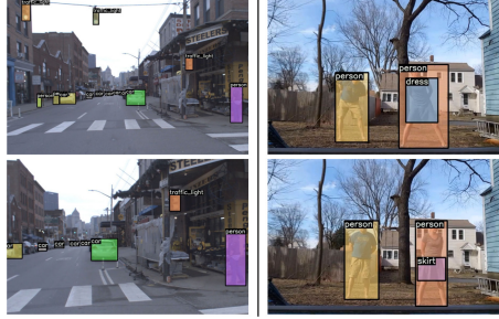
Fig. 4. SORT qualitative results, showing (left) a successful tracking result, and (right) a failure case due to semantic flicker between similar classes, suggesting that large-vocabulary tracking on TAO requires additional machinery.
