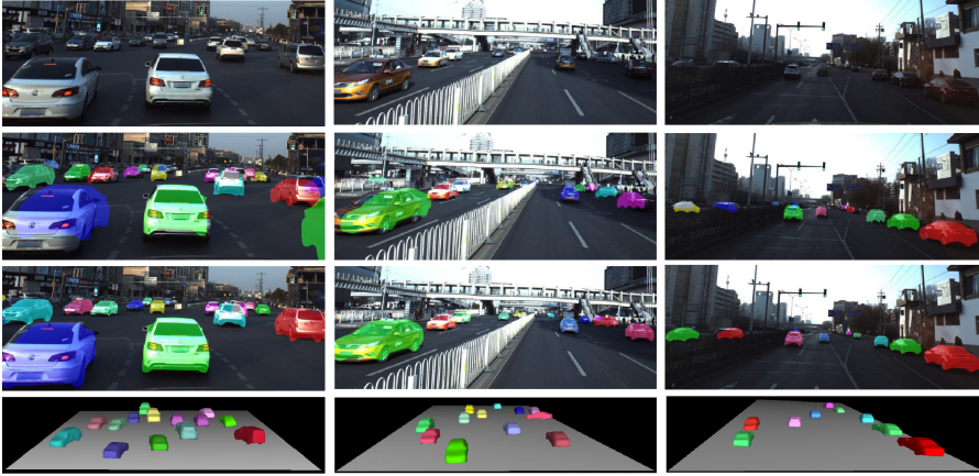
Fig. 5. Qualitative comparison on the ApolloCar3D test set of different approaches by rendering 3D mesh output projected onto the input 2D image. The first row are the input images, the second row is the result of Direct-based [48] and the third row is predicted by our GSNet. The bottom row shows the reconstructed meshes in 3D space. Corresponding car instances are depicted in the same color. (Color figure online)
