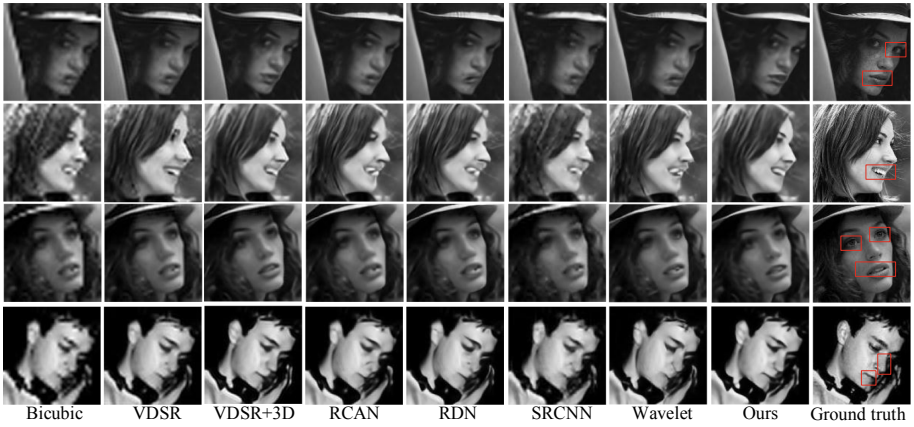
Fig. 5. Comparison of state-of-the-art methods: magnification factors \times 4 and the input resolution 32 \times 32 . Our algorithm is able to exploit the regularity present in face regions rather than other methods. Best viewed by zooming in on the screen.
