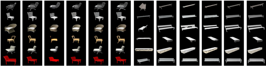
Fig. 2. Comparison of “chair, bench” category on ShapeNet with a single 2D input. From left to right: 2D-input, ground-of-truth, MV3D [71], AF [85], pose-supervised VIGAN [79], Our unsupervised AUTO3D. AUTO3D is comparable to the pose-supervised VIGAN and significantly better than MV3D/AF.
