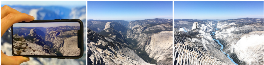
Fig. 9. An iPhone application (in the left) is used to capture the photograph (in the middle) for which precise camera pose is estimated using our method. The estimated camera pose (in the right) is used to augment the query photograph with contour lines (white) and rivers (blue). (Color figure online)
