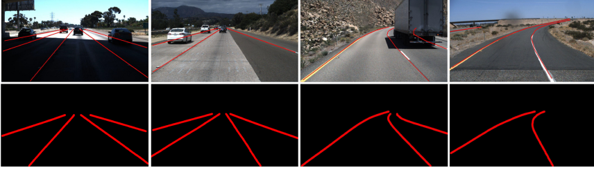
Fig. 6. Visualization of Failure cases. Top Row: images with ground truth. Bottom Row: the results produced by our PRNet. Here the four categories of failures are shown from left to right, including initial retrieval point missing (IRPM), wrong prediction of initial retrieval points (IRPW), inaccuracy of polynomial regression (PRI), and inaccuracy of height regression (HRI).
