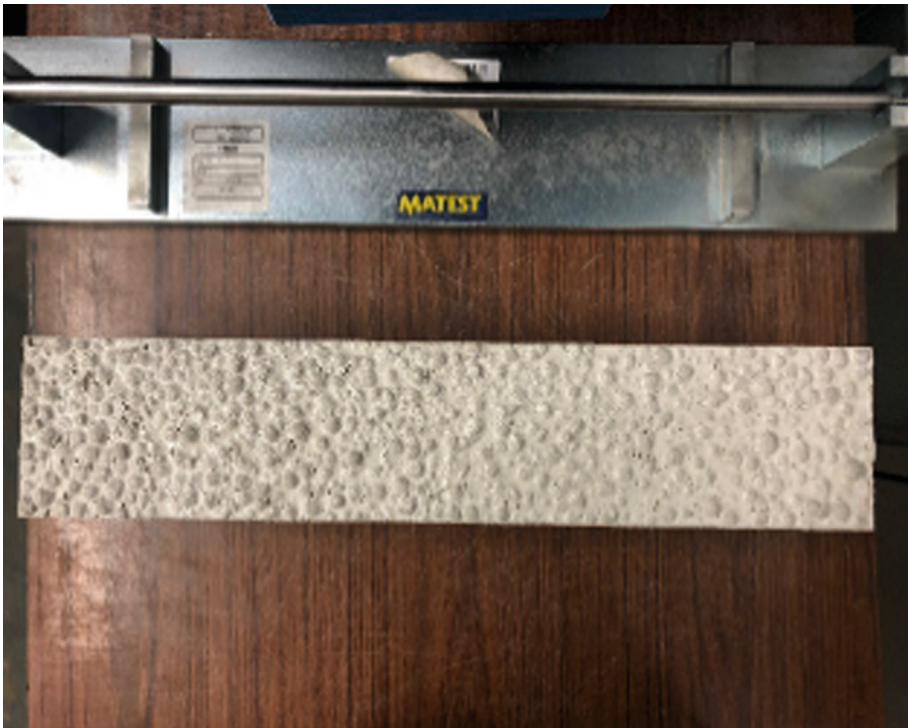
Fig. 2. Concrete specimen about to be housed in the measuring apparatus
