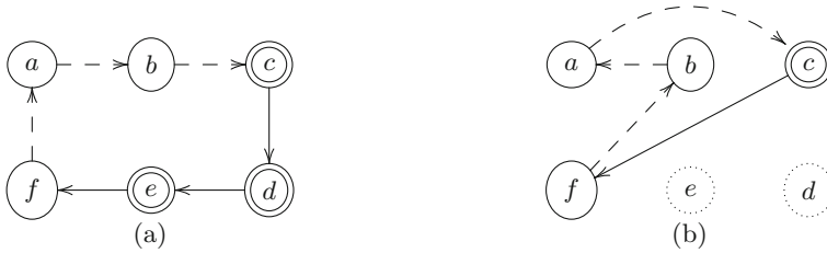
Fig. 1. Visualization of circuit aggregation via short-circuiting. The current solution (a) has realized nodes shown in double circles. Nodes d and e can be removed as garbage and node c is short-circuited to point at f , but must remain since (b) some non-garbage node will point at it, in the next session.
