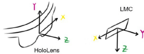
Fig. 8. HoloLens and LMC coordinate reference systems
