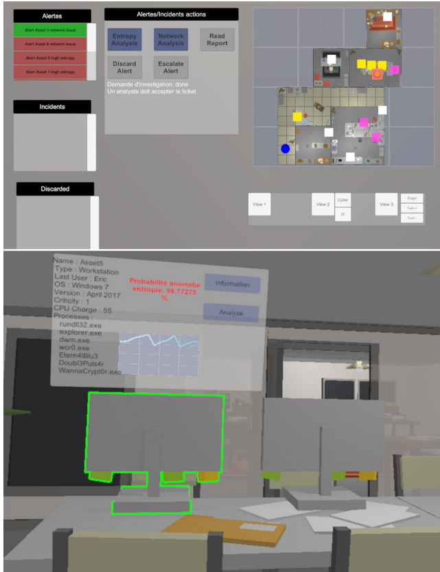
Fig. 3. Examples of visualizations developed from our activity analysis: a 2D monitoring dashboard (TOP) and an immersive interface (BOTTOM).
