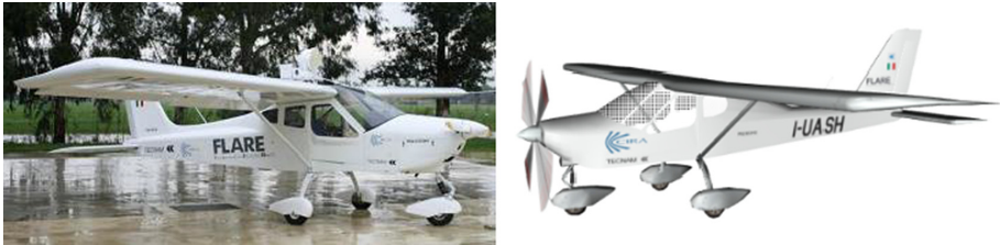
Fig. 9. The CIRA FLARE flight testbed (TECNAM P92-S Echo) and its 2500-triangle virtual counterpart in the HSTT application.
