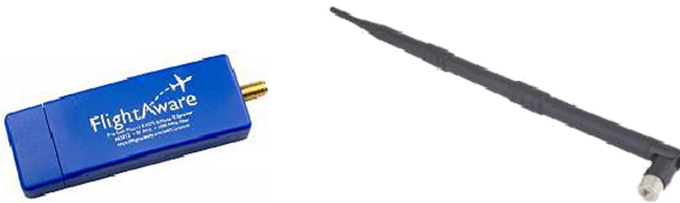
Fig. 3. USB SDR dongle for receiving ADS-B signals [20] (left), and related 9 dBi antenna [21] (right) - objects not in the same scale.
