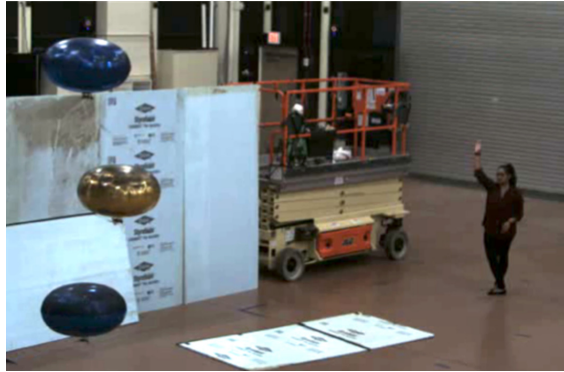
Fig. 2. A user makes the Up gesture, which is the vertical formation command gesture. This tells the agents to go to the same x and y location but be separated in altitude ( z ) by 1.5 m between each agent.
