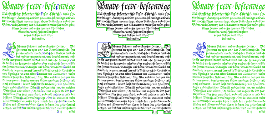
Fig. 3. The left image shows the prediction of the contour classifier. The image in the middle depicts the text and image regions detected by the post-processing algorithm. The rightmost image shows the corrected prediction when using the results of the post-processing. Contours / regions belonging to the text class are colored in green while non-text elements are illustrated in blue (Color figure online).
