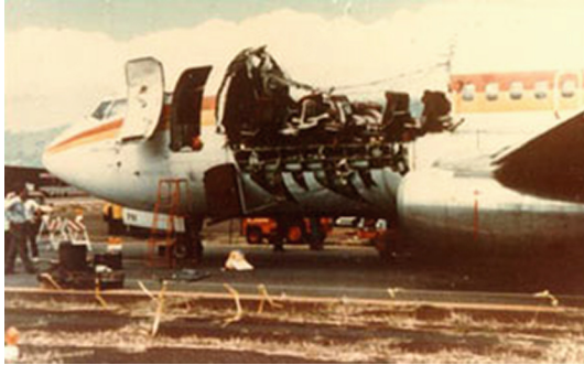
Fig. 1. Aloha airlines flight 243 damage (Source federal aviation administration)
