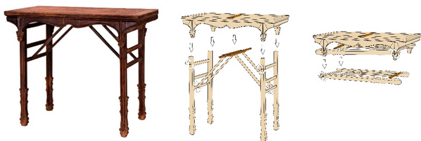
Fig. 3. The mortise and tenon structure of high legs of the elm high and low dual-purpose table
