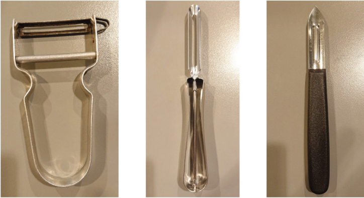
Fig. 1. The three potato peelers used, namely the y-peeler with flexible blade (left), vertical with flexible blade (middle) and vertical with fixed blade (right).
