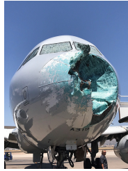
Fig. 4. American airlines, airbus 319 DAMAGED by hail (Source, courtesy of American airlines)
