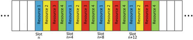
**Fig. 15.21** Illustration of DL-PRS resource repetition factor and DL-PRS resource time gap for a single instance of the PRS resource set
