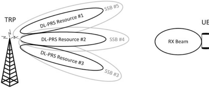
**Fig. 15.20** Illustration of quasi-colocation (QCL) indication for a “fixed” UE RX beam
