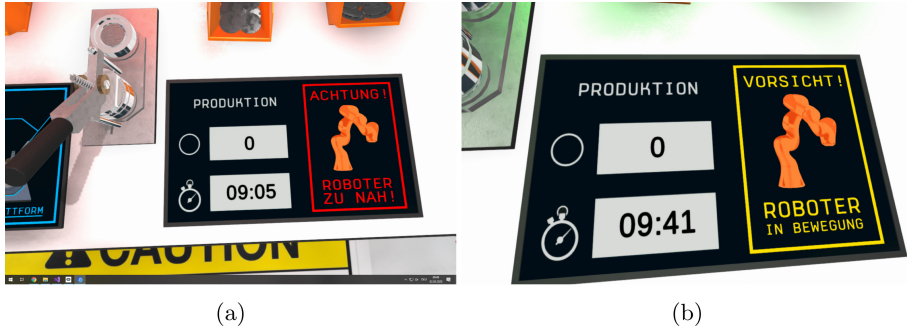
Fig. 4. Display with additional explanation: (a) Attention! Robot too close, (b) Caution! Robot is moving
