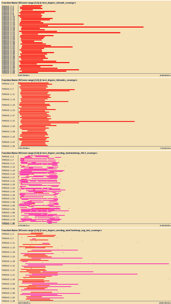
Fig. 4. Traces for SpMV when applying taskloop with 1 (first) and 4 chunks (second) per core, taskloop + nesting with th = 25\% L2 (third) and th = avg\ nnz per chunk (fourth) optimizations to taskloop approach.
