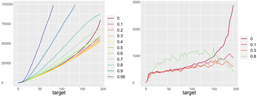
Fig. 4. Left: Average fixed-target running times of the (50 + 50) GA with uniform crossover and standard bit mutation on LEADINGONES in 200 dimensions, for different crossover probabilities p_c . Results are averages of 100 independent runs. Right: Gradient of selected fixed-target curves.
