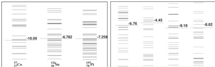
Fig. 4 (Left) Single particle energy levels of nuclei from HFB calculations using a Skyrme EDF (SkO') [20–22]. (Right) Results of HFB calculations for N = 76 and three realizations from the RS model. Dotted lines represent the Fermi surface. Figure adapted from [19]
