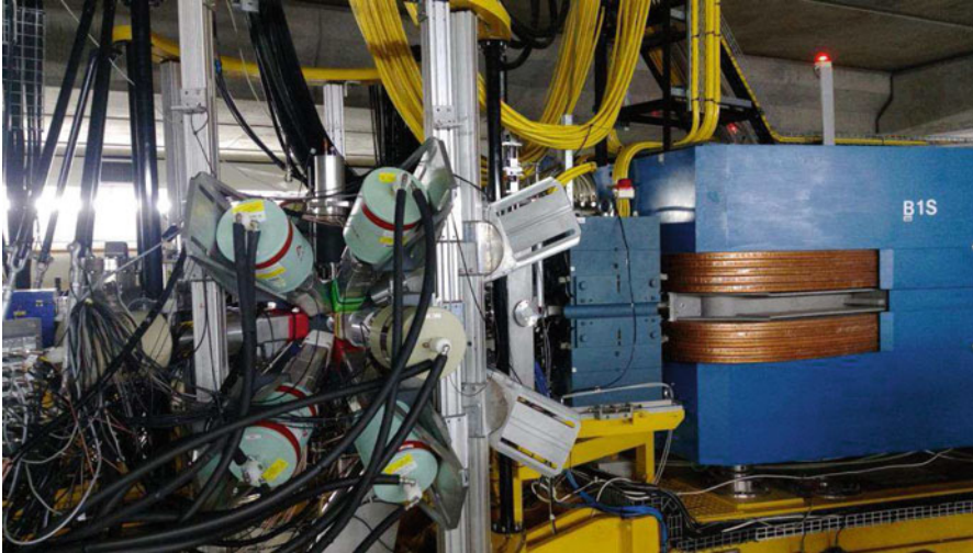
Fig. 1 Coupling Clover \gamma -ray detectors to the K600 magnetic spectrometer. Visible on the left are Clover detectors around the scattering chamber and on right is the first of two dipole magnets of the K600
