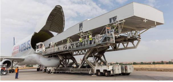
Fig. 2. The transportation jig during loading at the Airbus Beluga.
