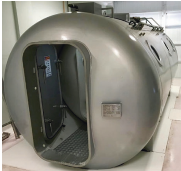
Fig. 64.13 Hyperbaric chamber 5 meters long and 2.20 meters in circumference can serve up to 8 patients per session. (Photo courtesy of Dr. Moacir Eduardo Armelin)
