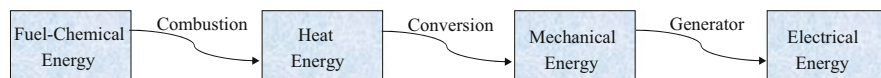
Fig. 1 A typical representation of the multiple conversions of energy required to electricity generation
