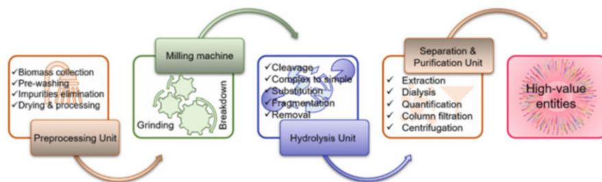
Fig. 1 Various key steps involved in the processing of biomass to high-value entities
