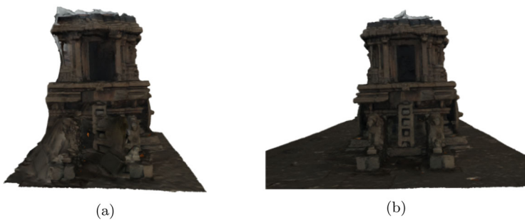
Fig. 9 (a) 3D model of Hampi obtained from images containing shadow. (b) 3D model of Hampi obtained after removing images containing shadow
