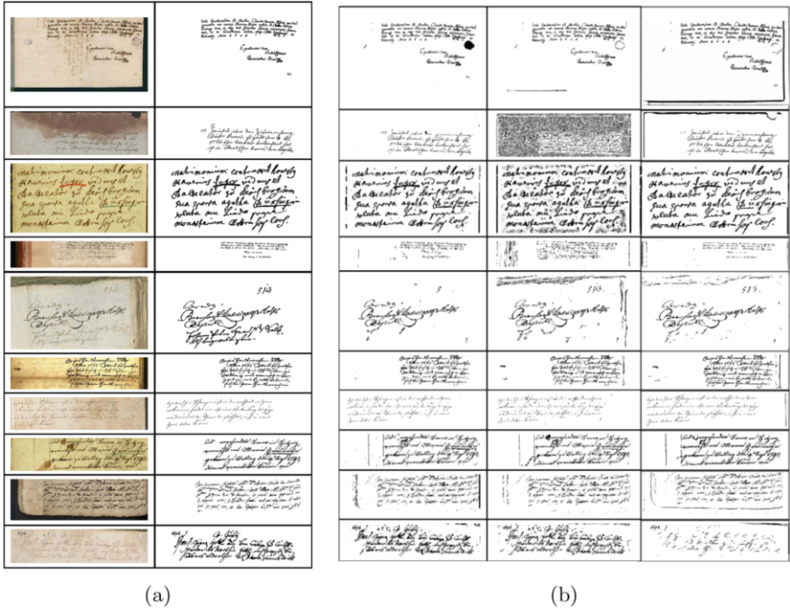
Fig. 15 (a) (Left to right) The result on H-DIBCO 2018 testing dataset, its corresponding ground truth, (b) binarization results on H-DIBCO 2018 testing dataset from (left to right) the winner algorithm, the algorithm that ranked in the second position, our method (Image courtesy of [12] for the first four columns)
