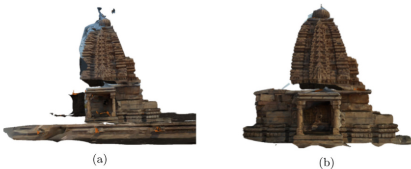
Fig. 8 (a) 3D model of Pattadakal obtained from images containing occlusion. (b) 3D model of Pattadakal obtained after discarding images containing occlusion
