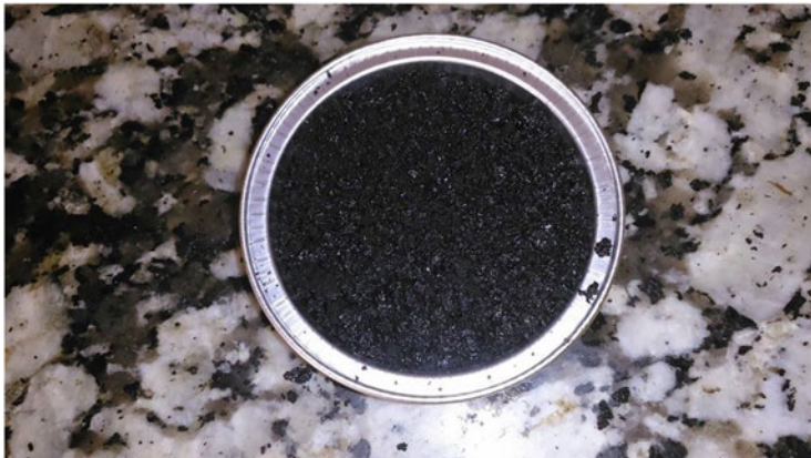
Fig. 9 Oily mud dries with 600°C
