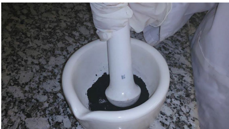
Fig. 10 Crusher mortar has agate
