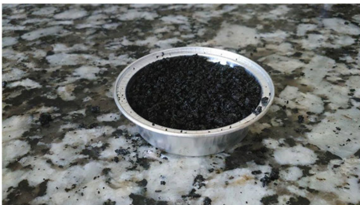
Fig. 8 Oily mud dries with 200°C
