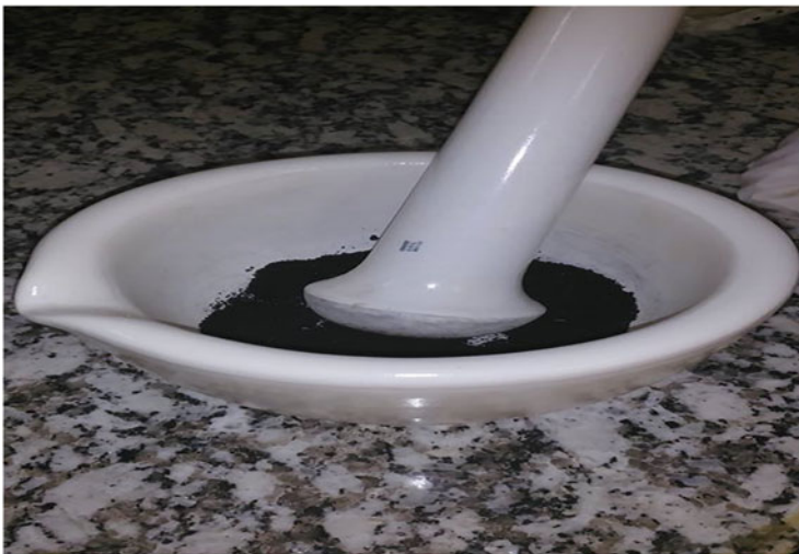
Fig. 12 Crusher with agate mortar and rammer oil
