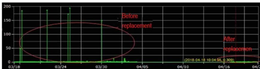
Fig. 123.8 The vibration data before and after the replacement of the bearing
