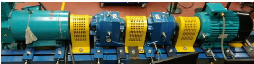
Fig. 117.9 Gear Run-to-fatigue Test rig
