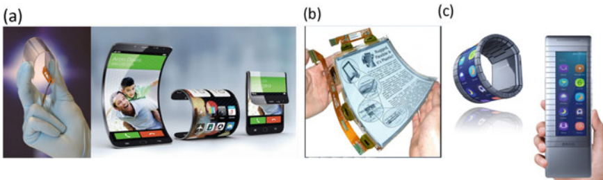
Fig. 14 Demonstration of flexible displays utilizing graphene technology [124, 126] in (a) and (b), while commercially available products such as the bendable smartphones produced by Moxi, a company based in China are now available [125] (c). Reprinted by permission from [125]. © 2014 Macmillan Publishers Limited (2014)
