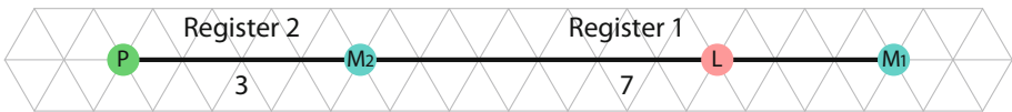
Fig. 2. A RAM simulator with the first register holding the value 7 and the second register holding the value 3
