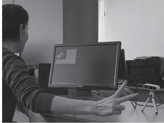
Fig. 6. Samples human hand gesture tracking from RealSense D435 sensor
