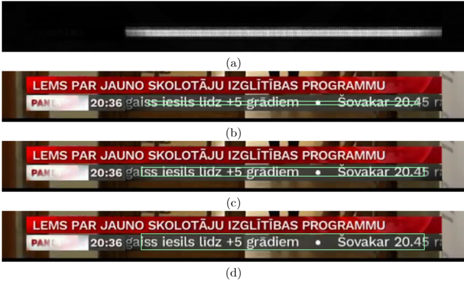
Fig. 2. Visualization of steps of ticker text localization for a section of the video containing a ticker. (a) Heat map of average change in brightness. (b) Initial window calculated in section “Guess Initial Text Position”. (c) Window after line-by-line expansion in section “Refine Guess”. (d) Window after expanding 1/3 to include possible diacritics and descenders in section “Expand Window for Diacritics”.
