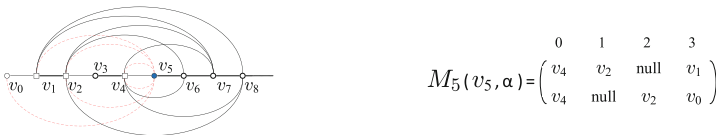
Fig. 3. A partial 2-page assignment of the edges in E_5 (left) and the corresponding crossing number matrix (right).
