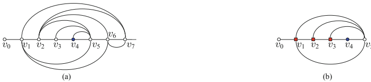
Fig. 2. An example on Edge-Pruning-1 from an original 2-page assignment of E_4 (a) to a simplified 2-page assignment (b).
